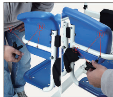
37. Fasten backrest onto seat frame tube, lock in corresponding holes with medium screws in sequence, tighten with hexagonal wrench.
