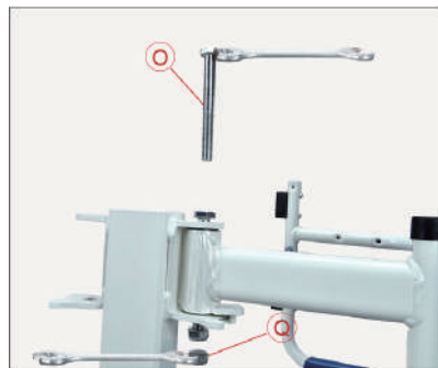
19. Insert the long screw into hole, lock with the nut.
