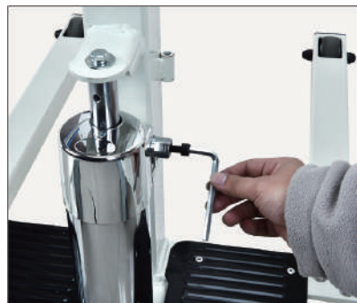
32. Take out the screw of hydraulic cylinder by wrench.
